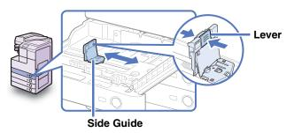
3 Squeeze the lever on the front guide. Without releasing the lever, slide the front guide backward or forward to align it with the mark for the desired paper size.
